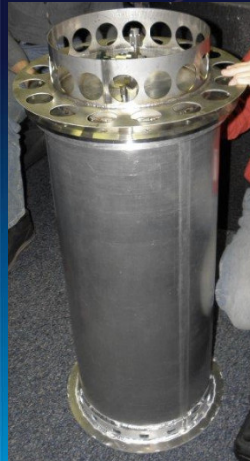
Al 6061-T6 Secondary Flange, Shell & Skirt
