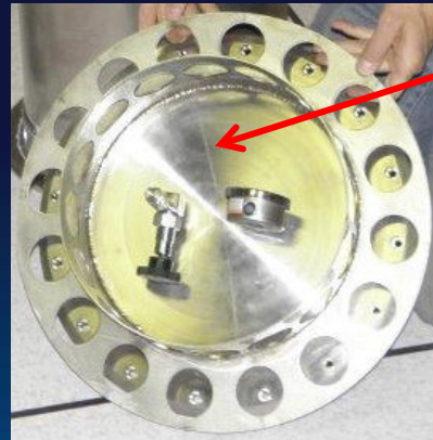
Al 6061-T6 Secondary Flange, Shell & Skirt
